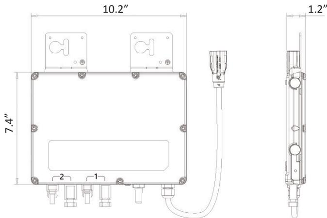
With its groundbreaking design and features, the YC600 is the pinnacle of microinverter technology. A single-phase, smart grid-compliant microinverter, the YC600 serves two modules with dual, independent MPPT. Zigbee wireless communication over a mesh network offers faster data speeds than PLC and a wider MPPT voltage range results in a greater energy harvest for homeowners.
